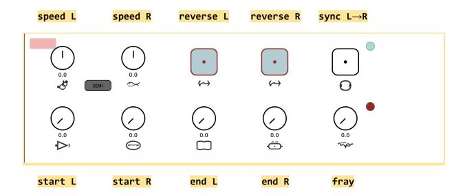
**speed L/R** changes the speed of the playheads for the left or right channel depending on the speed mode selected. To the left it slows down, to the right it speeds up. The toggle button creates a phase inversion to make the buffer wider in the stereo field.
